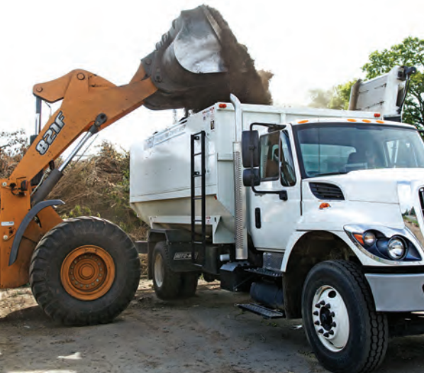
A specialty truck (Roto-Mix) is loaded with biosolids to which wood waste is later added.
