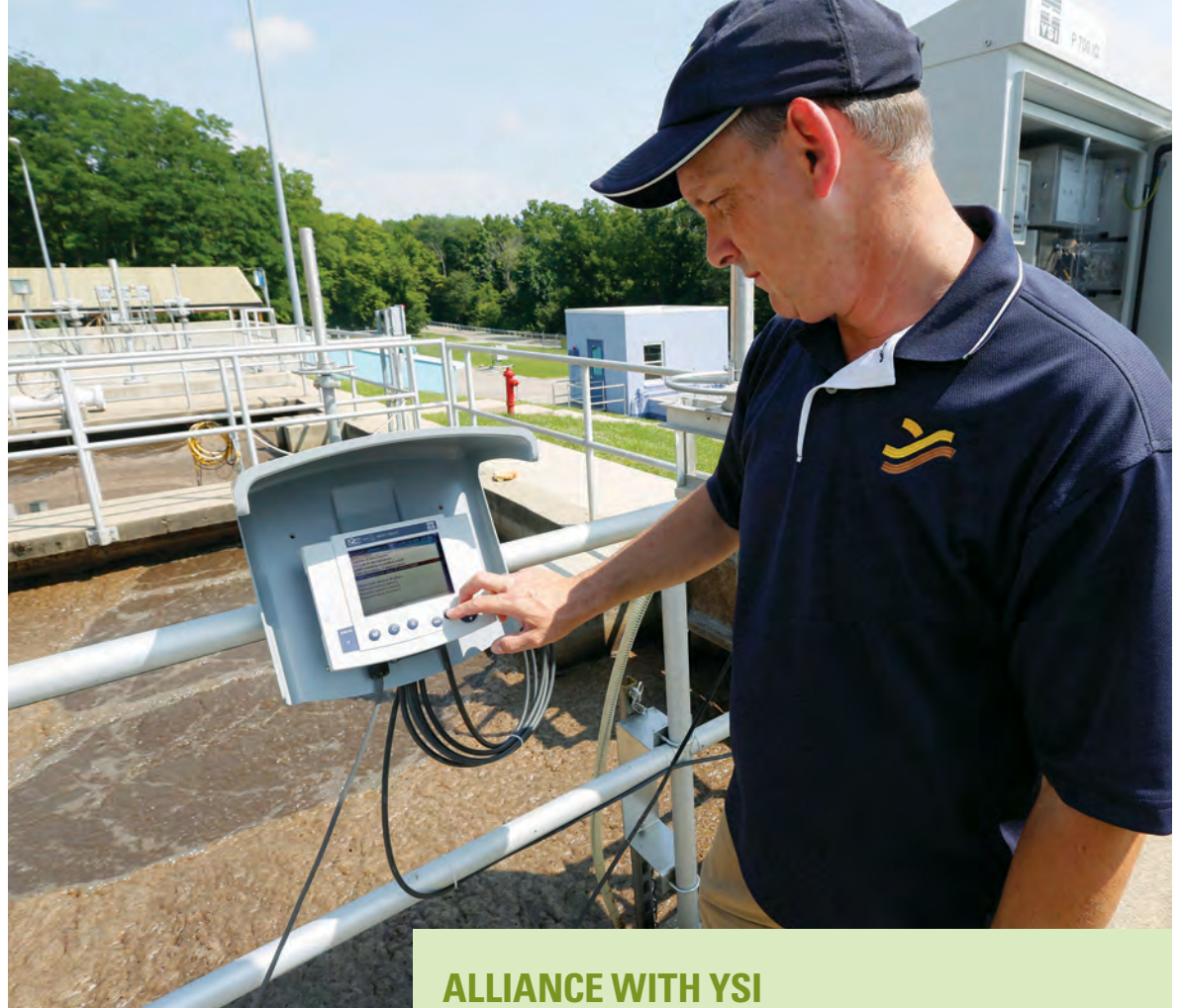
Bates uses tools including this YSI IQ SensorNet 2020 XT to monitor water quality.
