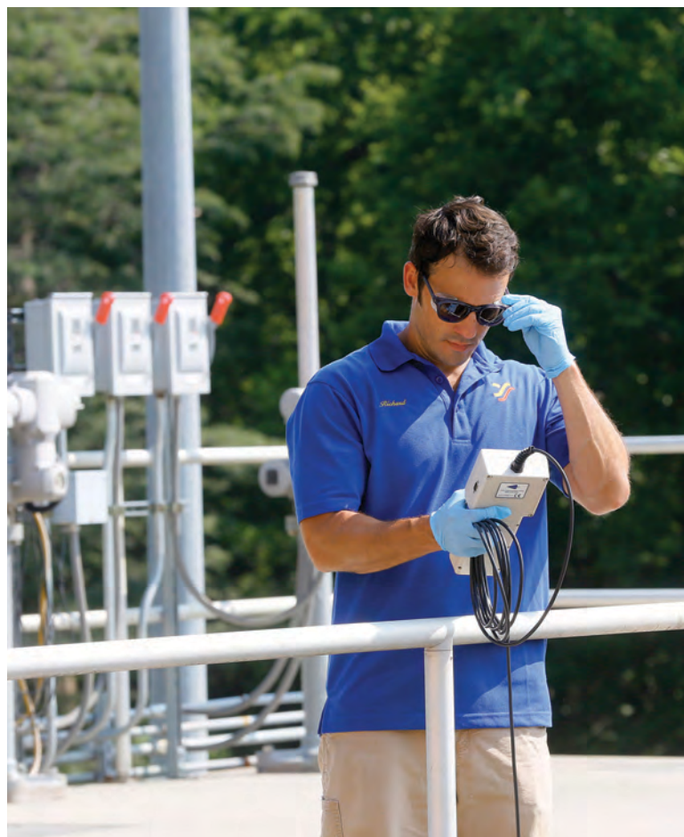
Operator Richard Stockton uses a suspended solids analyzer (InsiteIG).
