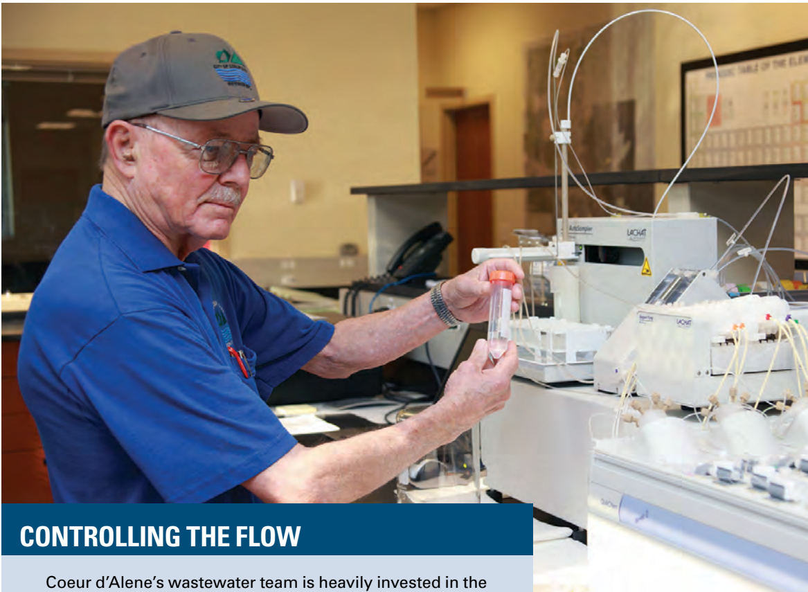
Sid Fredrickson works with an auto-analyzer for phosphorus and nitrogen. Nutrient removal is essential to the Coeur d'Alene plant's process.
