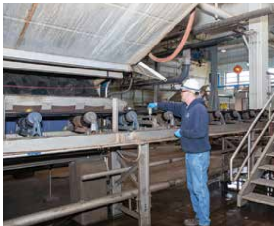
Biosolids dewatered on an Ashbrook belt filter press (Alfa Laval) are incinerated or land-applied.
