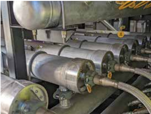
Membrane filters are part of the Unison Solutions system to convert biogas to renewable natural gas.
