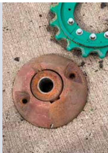
Old-style bearings that had been installed in the grit channel were removed and replaced.
