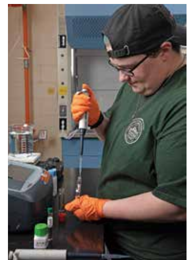
Kate Preston uses a Hach DR3900 spectrophotometer and a Hach DRB200 incubator for the TNT800 test.
