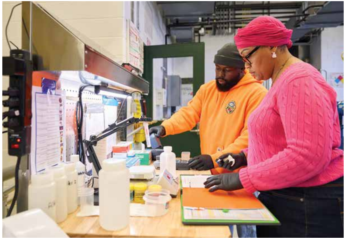
Oberton and Devene Spence, operator, use a Hach SL1000 analyzer to test water samples.
